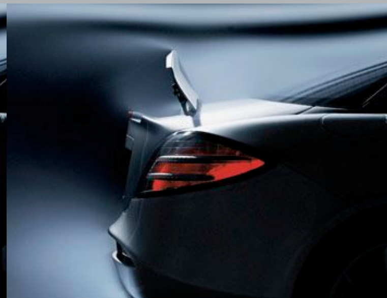
Automatic 65° position on emergency braking
