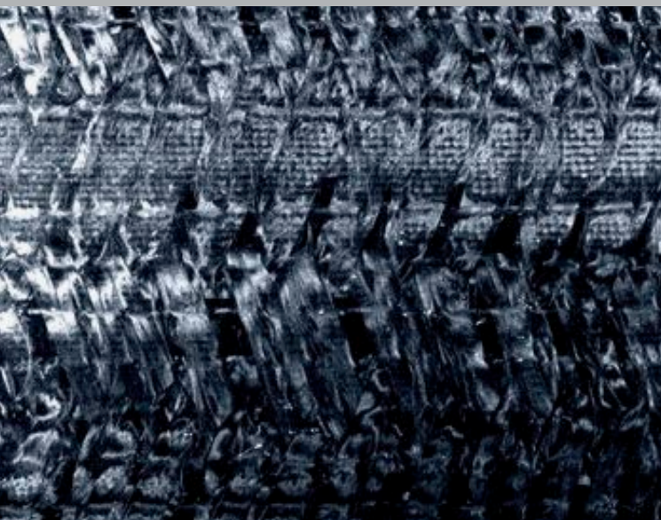
Detail of carbon-fibre composite structure
