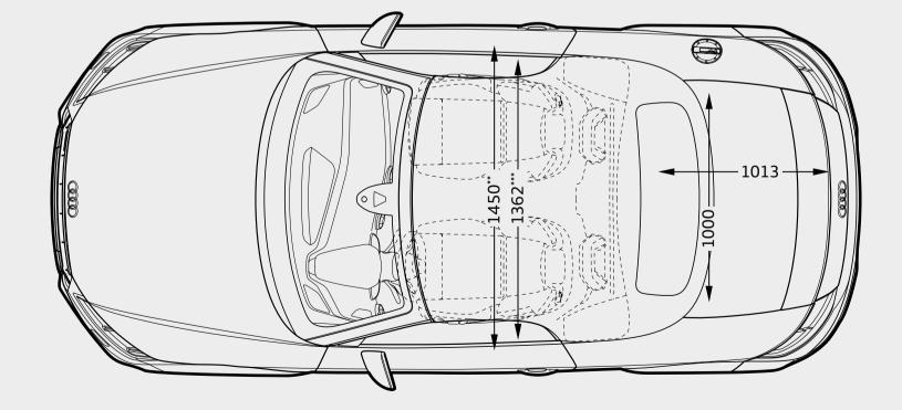
Dimensions in millimetres. Optional equipment may affect dimensions. Dimensions were measured with vehicle at unladen weight, ground clearance measured with vehicle carrying its maximum load. Turning circle approx. 11m. \*Maximum headroom. \*\*Elbow room width. \*\*\*Shoulder room width.
