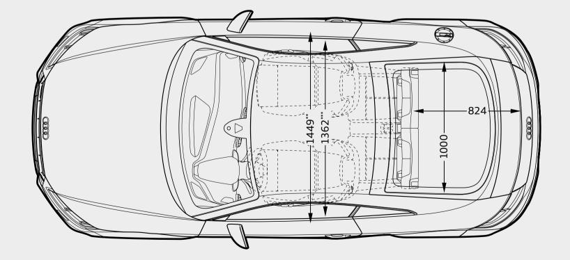
Dimensions in millimetres. Optional equipment may affect dimensions. Dimensions were measured with vehicle at unladen weight, ground clearance measured with vehicle carrying its maximum load. Turning circle approx. 11m. \*Maximum headroom. \*\*Elbow room width. \*\*\*Shoulder room width the VDA standard test method using 200 x 100 x 50mm blocks.
