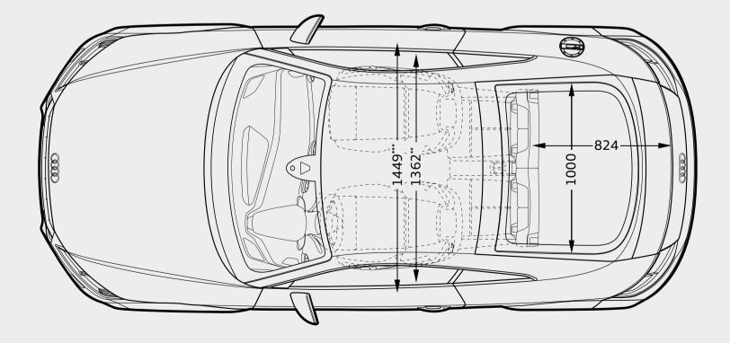
Dimensions in millimetres. Optional equipment may affect dimensions. Dimensions were measured with vehicle at unladen weight, ground clearance measured with vehicle carrying its maximum load. Turning circle approx. 11m. \*Maximum headroom. \*\*Shoulder room width. \*\*\*Elbow room width.
