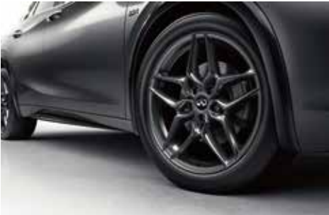
19" LIGHT ALLOY WHEELS WITH 5 DOUBLE-SPOKES, 235/45R19 RUN FLAT TYRES
