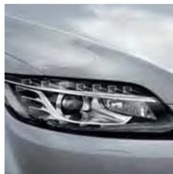
Xenon Plus headlights with LED daytime-running lights
