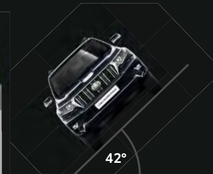
Limit angle of vehicle turnover
