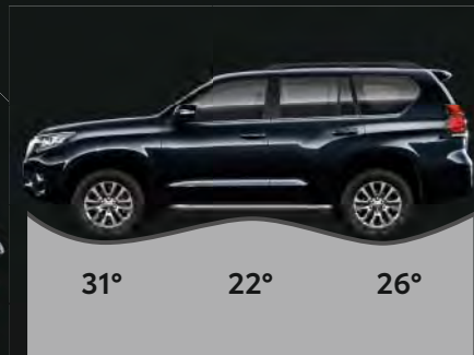
Approach, ramp break-over and departure angles
