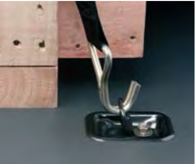
Load tie-down eyes Anchorage points throughout to secure loads.
