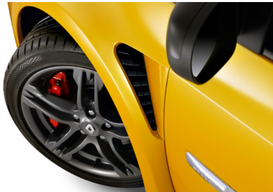
The extractor vents behind the front wheels reduce turbulence and enhance the car's aerodynamics.
