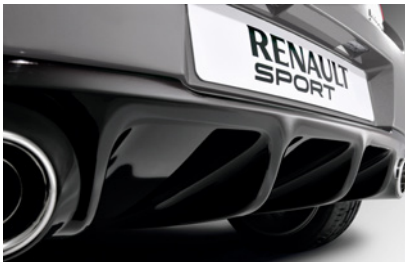
Rear diffuser derived from Formula 1 aerodynamics. Twin chrome exhausts are integrated into the diffuser.
