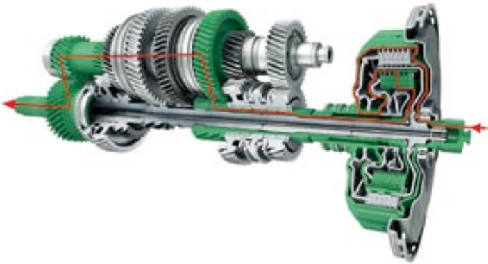
Power flow in 2 nd gear
