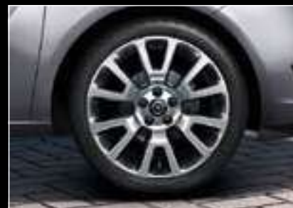
OPC Line alloy wheel, 7,5 J x 18", 6-V-spoke bi-colour design, tyres 225/40 R 18 (RT1). 10
