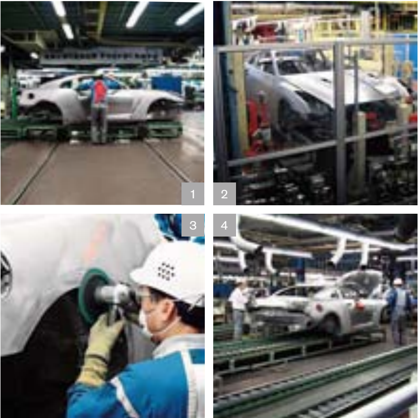
1_ Every GT-R receives a high degree of hand assembly and finishing. 2_ A grueling shake test verifies the quality of its many welds, helping ensure long-term durability. 3_ Hand-finishing of body panels creates a true work of art. 4_ “Jigs” or fixtures – a technique learned from racing – are used to hold body panels and components precisely in place during assembly.
